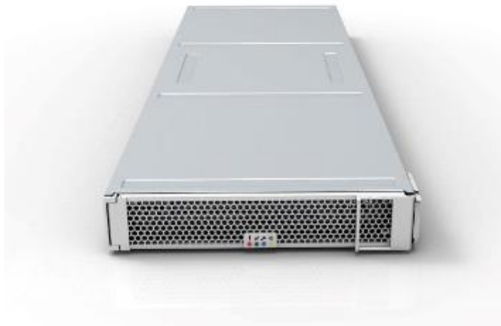
Slika 1.6 NSU – Network Sled Unit
