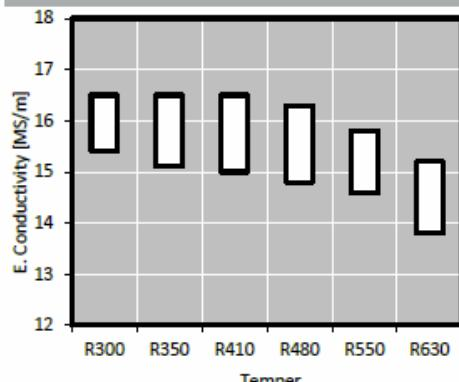
Electrical conductivity is strongly influenced by chemical composition. A high level of cold deformation and small grain size decrease the electrical conductivity moderately. Minimum conductivity level can be specified.
