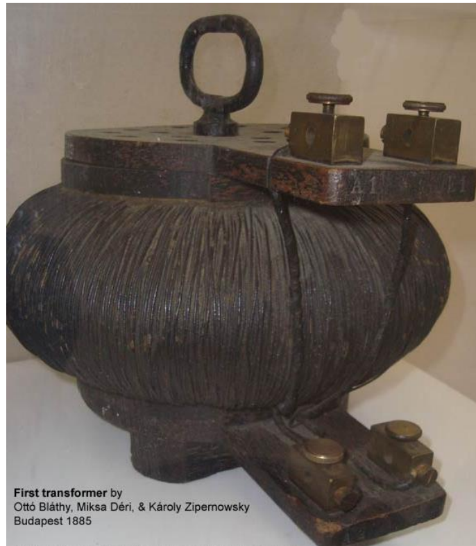
Slika 2. 2: ZBD transformator (izvor: https://basiceletrical.blogspot.com/2012/12/definition-of-transformer-transformer.html )
