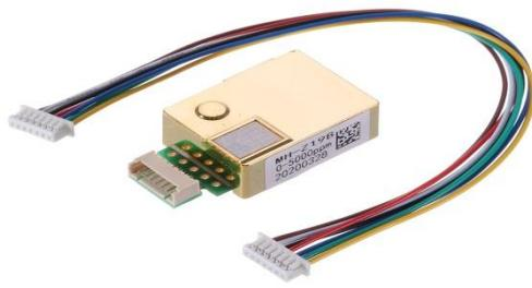
Slika 4.4 MH-Z19 infrared gas sensor
