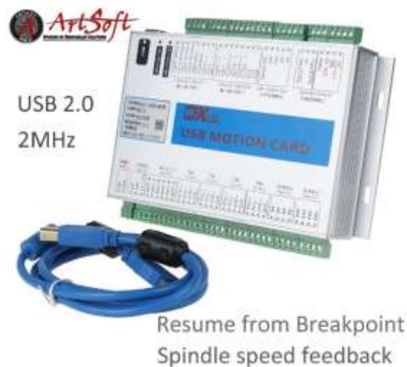
Slika 4.11 - UCONTRO Mach3 USB 4 Axis CNC Motion Control Card Breakout Board 2000 KHz, 2 MHz. [51]
